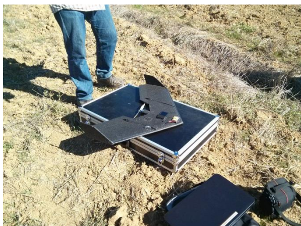
Figur 2. Fastvingedrone. Sensefly, Siena, 2013. Fotograf ESM.
