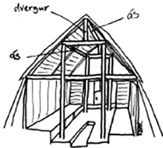
Fig. 4. Construction of a Viking Age hall from Gunnell (2004). By Karen Bek-Pedersen. Courtesy of Terry Gunnell.
